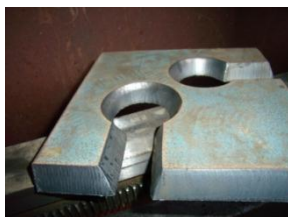
Cutting for bevel of steel plate
