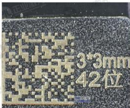
1. UV laser engraving QR code on steel stiffener of FPCB, QR code's size is 3mm×3mm.
