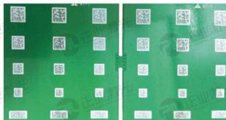
8. UV laser engraving QR code on PCB
