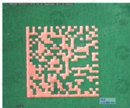
4. Fiber Laser engraving QR code on green oil of PCB, QR code's size is 3mm×3mm
