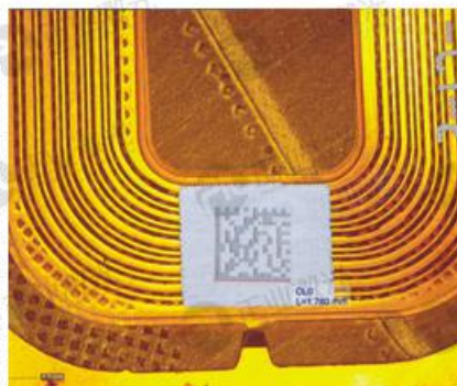
2. UV Laser engraving QR code on white oil of FPCB, QR code's size is 1.7mm×1.7mm..
