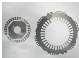
Active cell (silicon steel sheet)
