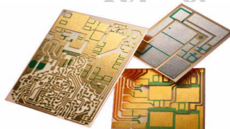
陶瓷 PCB Ceramic PCB
